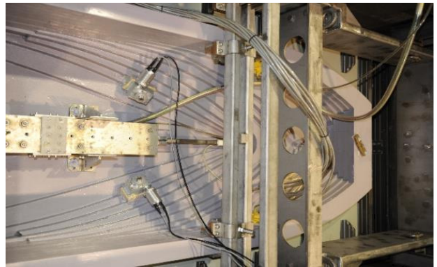
Fig. 4 Angular control system of vortex generator
