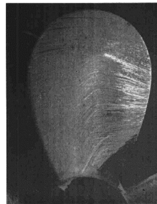
Fig. 15 Result of paint test for POW test(Kuiper, 1981)
