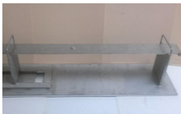
Fig. 12 Load cell structure of simply supported beam type subjected to end vertical downward load
