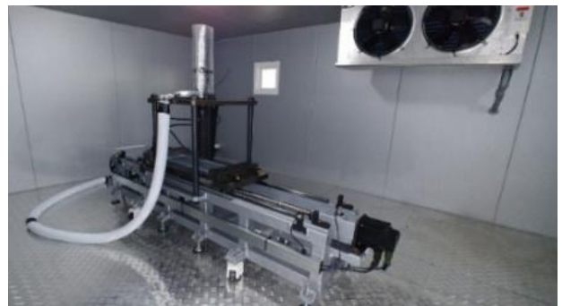
Fig. 3 Ice friction/abrasion tester in cold room
