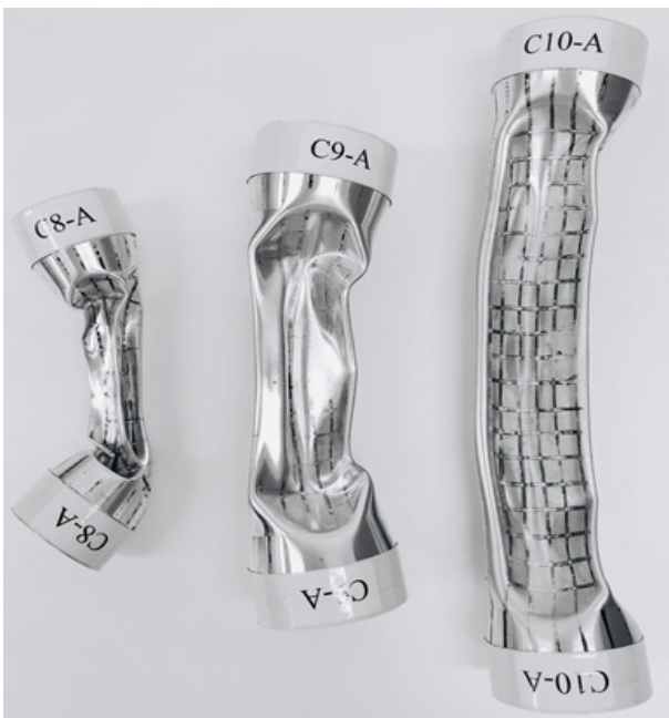
(a) Longitudinal deformed shape
