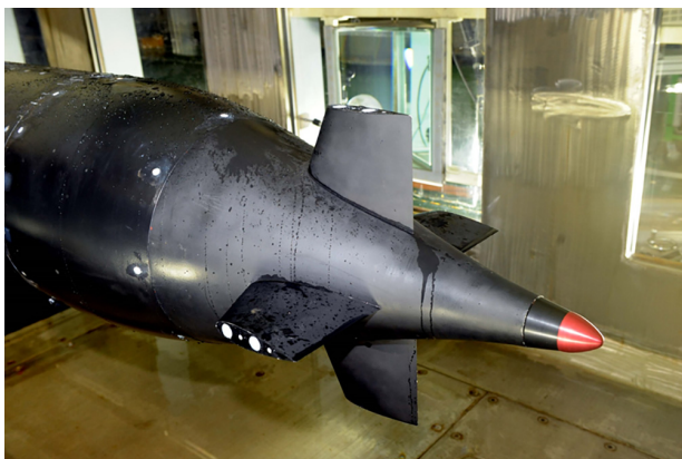
Fig. 6 Installation for the resistance test
