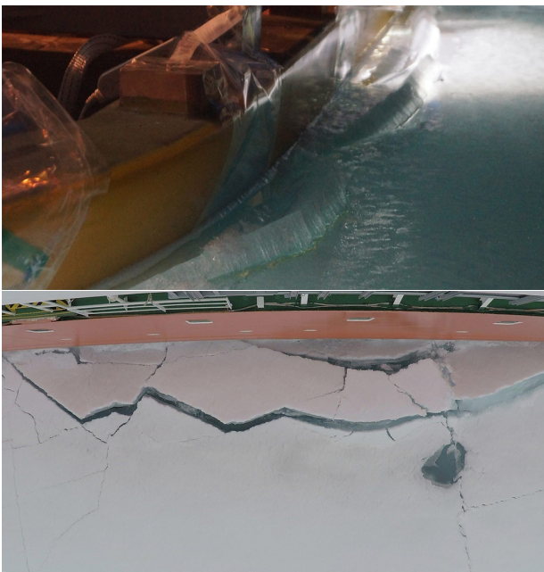
Fig. 14 Comparison of icebreaking pattern between model-scale and full-scale for the Korean icebreaking research vessel Araon
