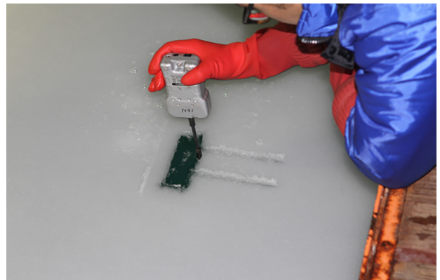
Fig. 7 Flexural strength measurement process by cantilever beam test(Jeong, 2016)
