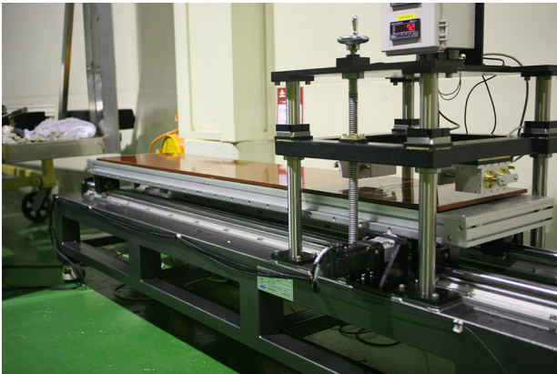
Fig. 3 An ice friction measurement device
