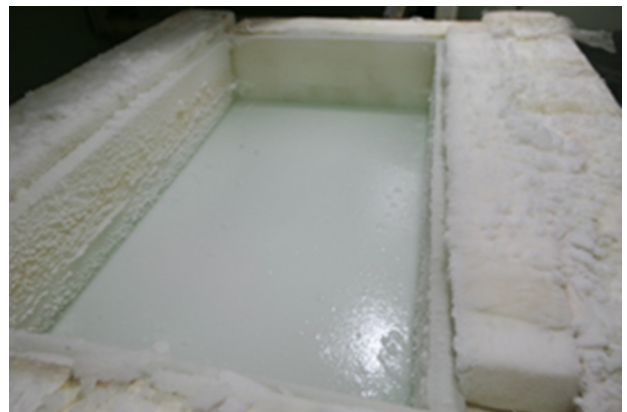
Fig. 2 PG/AD model ice sheet in the cold room facility
