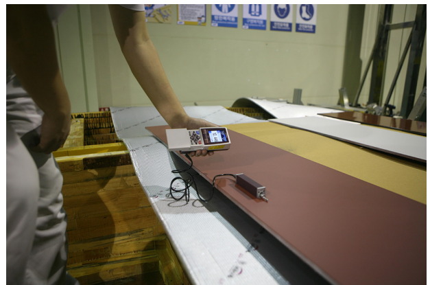
Fig. 4 A surface roughness measurement device
