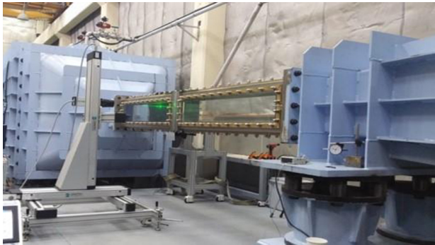
Fig. 1 High-speed cavitation tunnel (HCT) in KRISO
