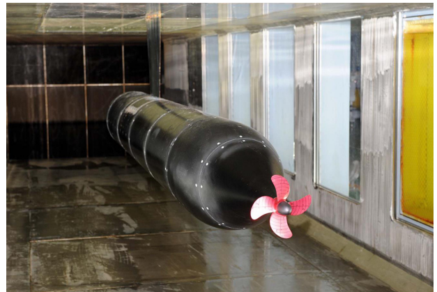
Fig. 8 Installation of axisymmetric body with propeller at test section of LCT
