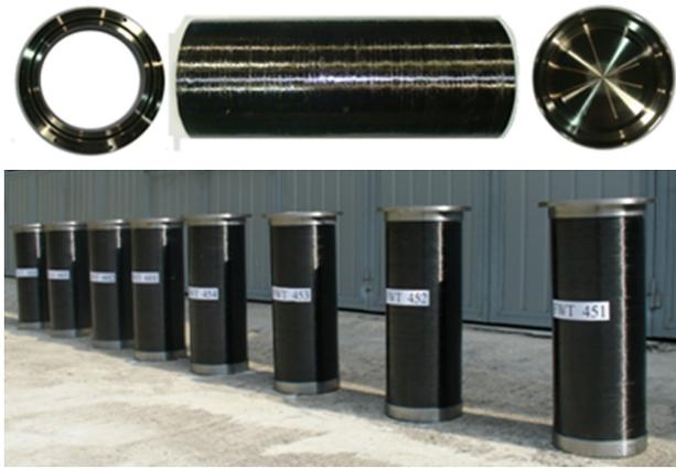
Fig. 3 Composite cylinder specimens for the hydrostatic pressure test
